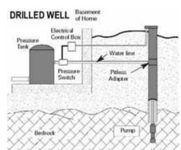
Drilled wells penetrate about 100-400 feet into the bedrock. Where you find bedrock at the surface, it is commonly called ledge. To serve as a water supply, a drilled well must intersect bedrock fractures containing ground water.
