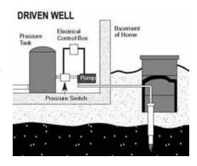
relatively inexpensive to install. Although deeper than dug wells, driven wells are still relatively shallow and have a moderate-to-high risk of contamination from nearby land activities.
